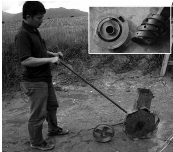
Figure 4. Manual wheel NT planter (Brazil) suitable for the sowing in line of various crops under limited soil mulch conditions.
