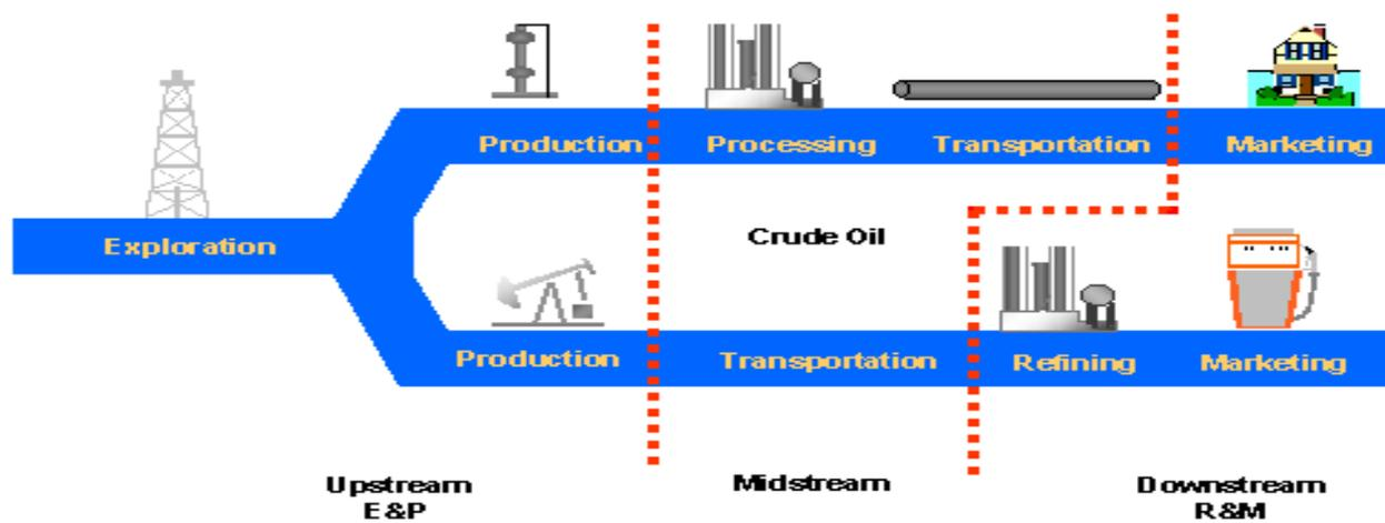
**Upstream work**, during the exploration and production process, accounts for over 75% of an oil company's capital output. The upstream process involves a large capital investment of equipment and technology to find the resource and to bring it to the surface. It consists of a number of sub-activities:<sup>486</sup>
