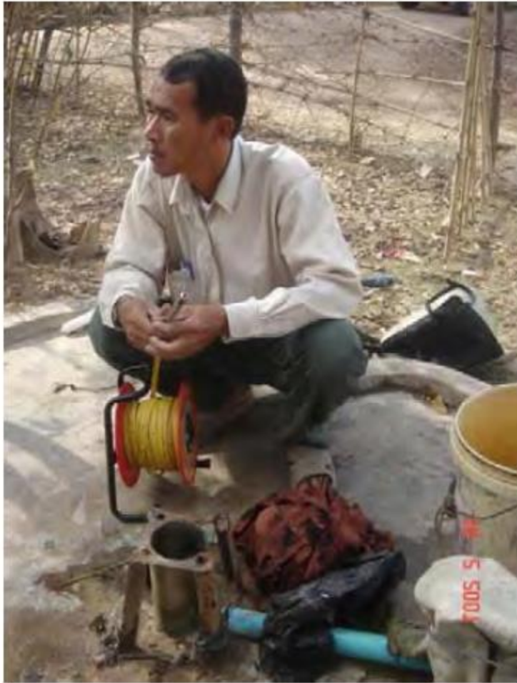
Measuring depth to groundwater at PRASAC monitoring well S4
