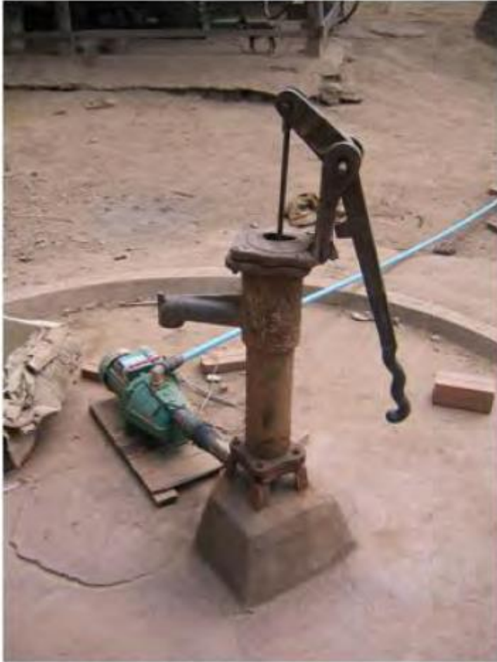
Suction pumps like this VN6 in Prey Veng will be out of service if the depth-to-groundwater falls below 6 m
