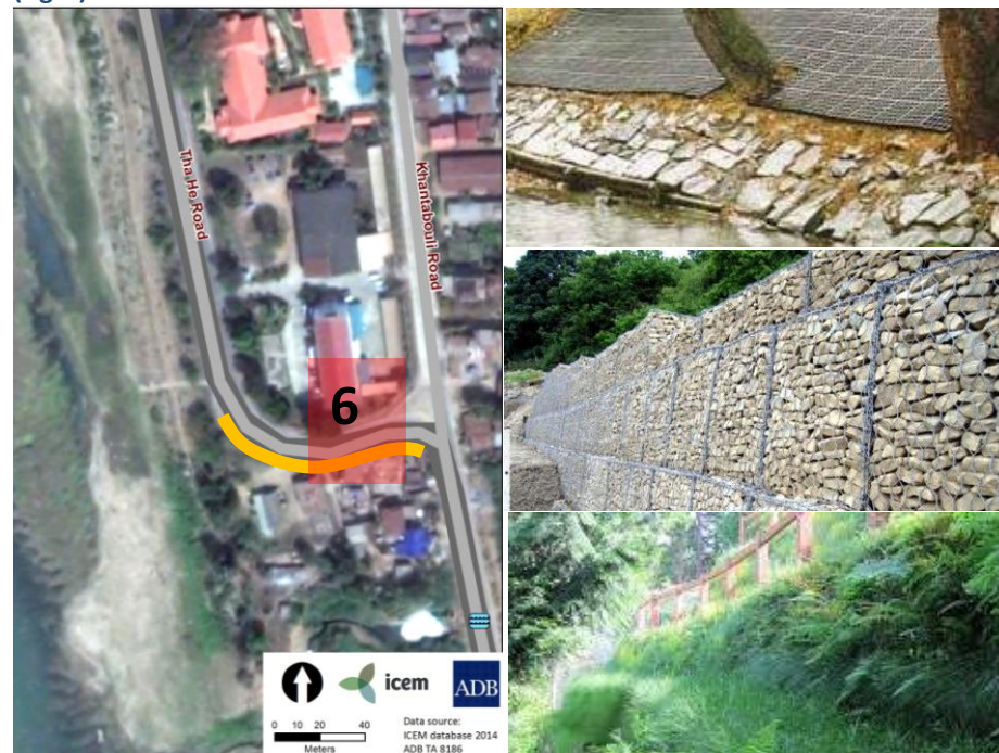
Figure 28: Dyke along Tha He road (left) with examples of slope stabilisation techniques (right)
