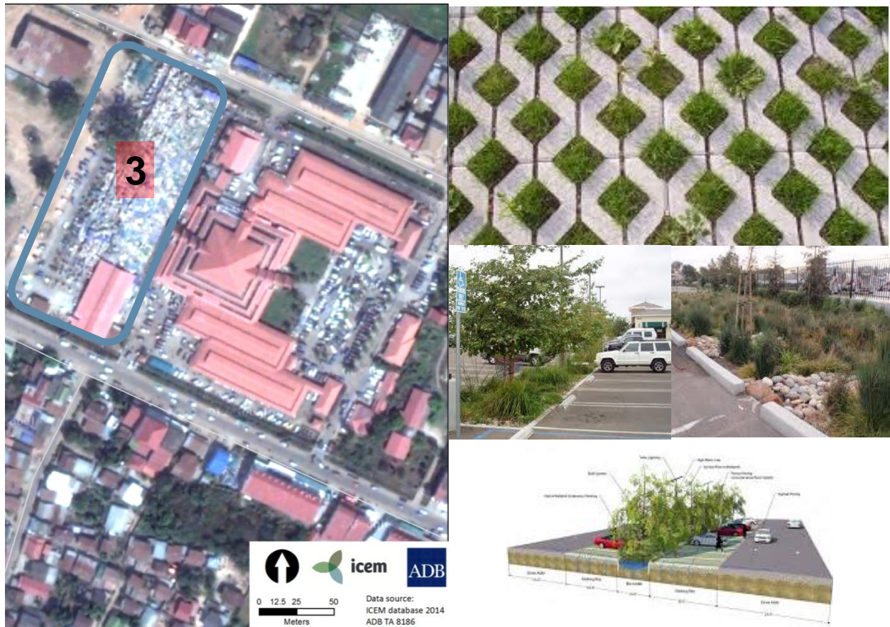
Figure 42: Parking area (left) with example of permeable paving, bio-swales and rain-gardens to increase infiltration and water purification
