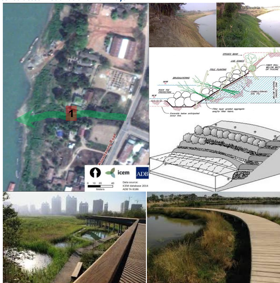
Figure 40: Mekong exit canal (left) – with examples of stabilisation and bio-engineering of canal banks and constructed wetlands and walkways
