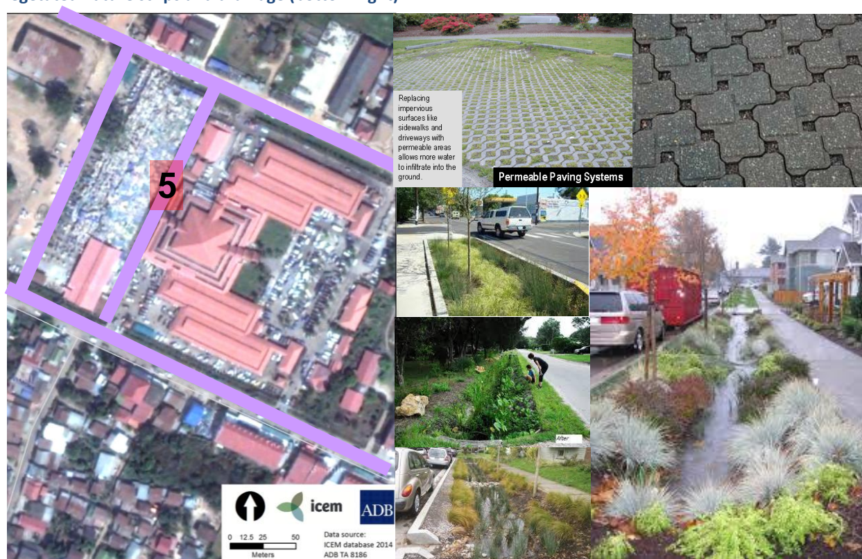
Figure 44: Walkways and footpaths around the market (left) with examples of permeable paving (top right), vegetated nature strips and drainage (bottom right)
