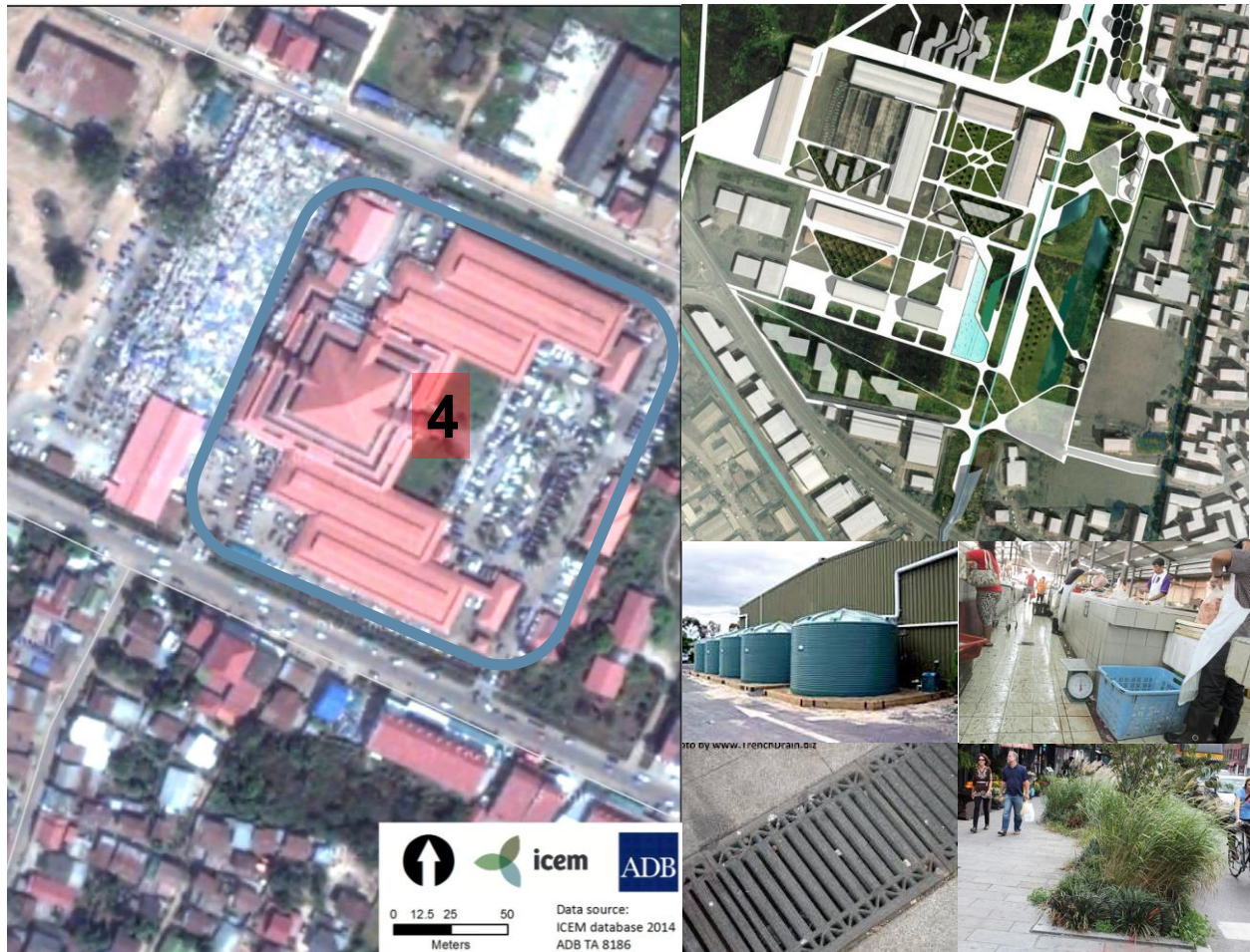
Figure 43: Savanxay Market (left) with examples of increased permeable surfaces (top right), waste collection and treatment area, rainwater collection, adequate drainage and bio-swales
