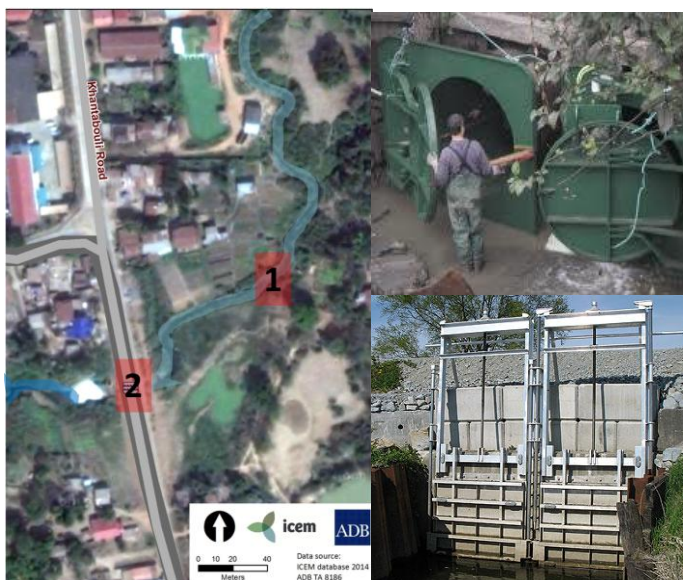
Figure 24: Flood gate (left at 2) with examples of more robust flood gates designed for manual operation (right)
