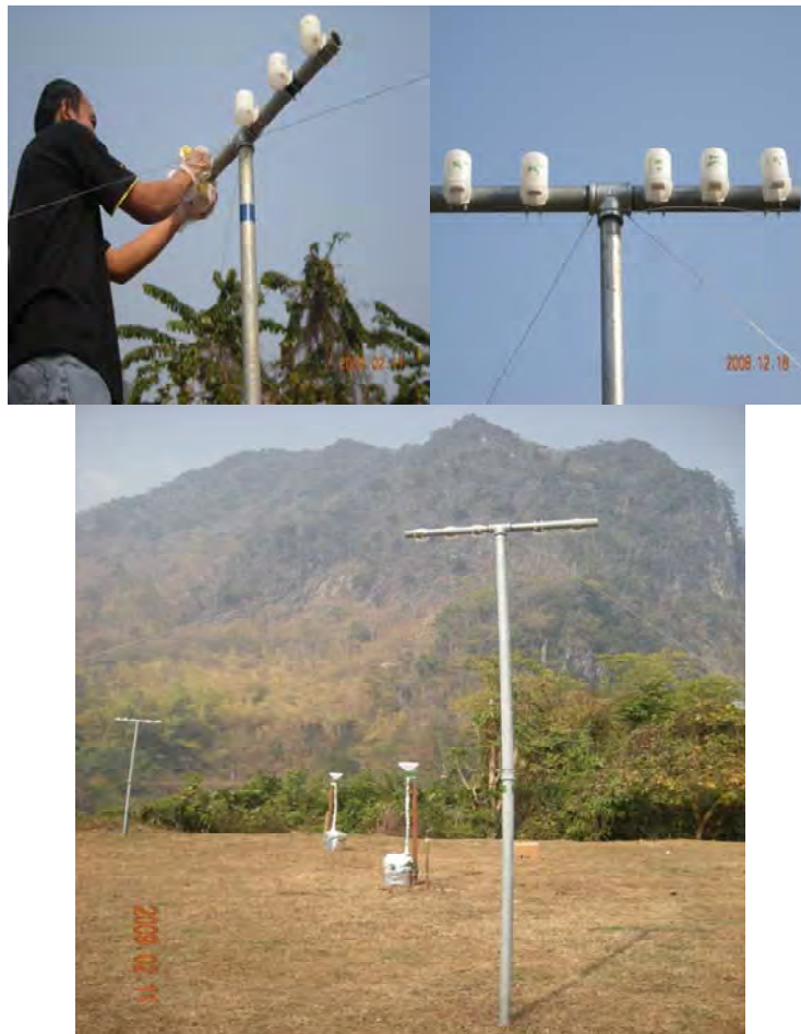
Figure 12.5: Gas measurements by Ogawa passive samplers
