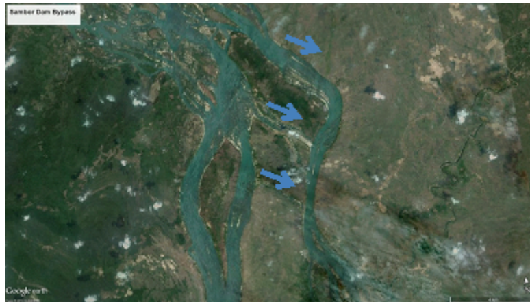
Figure 6.2.2. Satellite image of the upstream end of the Sambor Alt_7 reservoir site, with blue arrows indicating natural spillways into the anabranch channel.
