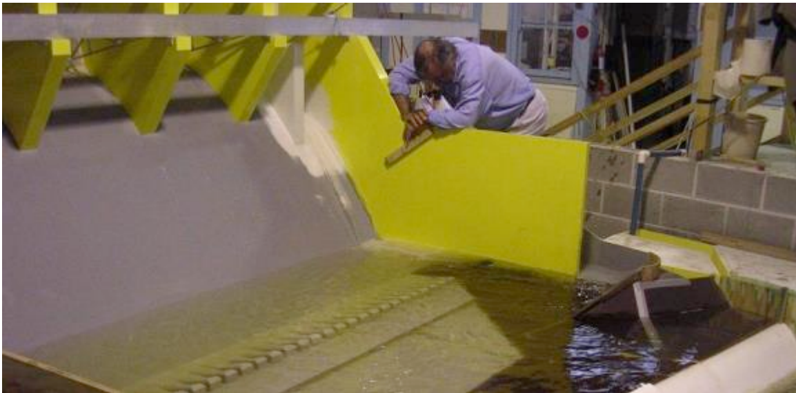
Figure 7.1.2. Example of a physical model of a 32m high dam and fishway in Australia that was used to determine entrance location and hydraulic conditions for the fishway. Scale is 1:20 but 1:10 is preferred.
