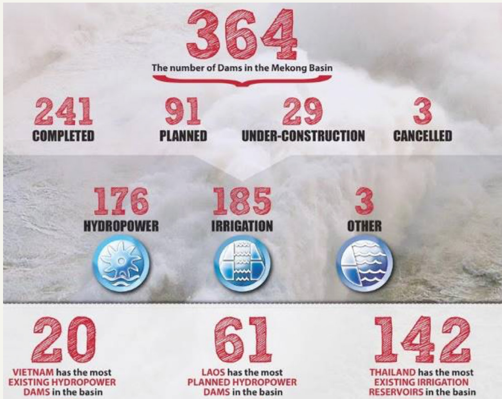
Figure 40: Overview of the large dams and their purpose in the Lower Mekong Basin. Source: CIGAR
