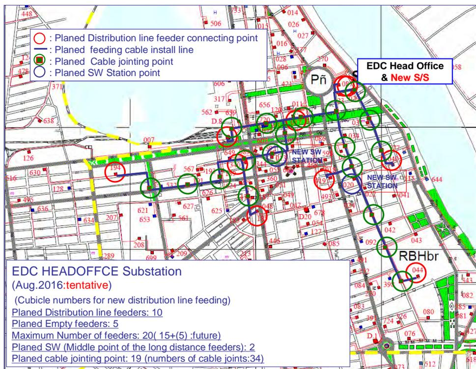
(a) Feeder line connection point, feeder line route and UG cable jointing points
