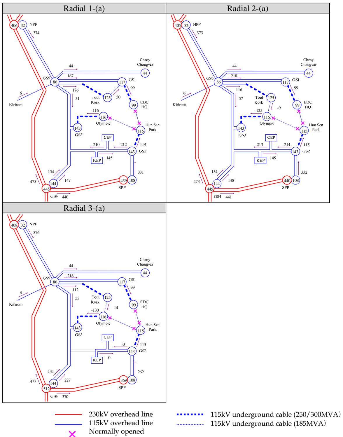
Figure 3. 23 Active Power Flow Diagram in Radial System Operation in 2020
