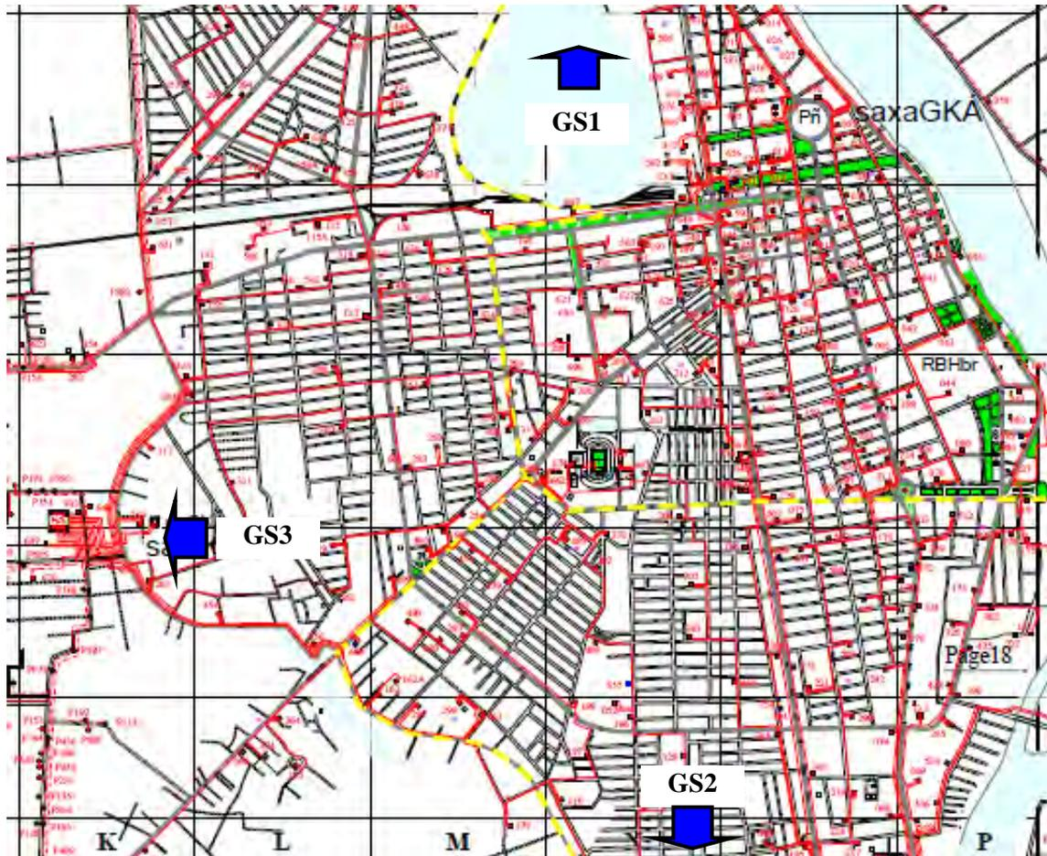
\*The yellow line almost expresses the load of each distribution substation's load allotment border, each distribution substation for the supply of electricity.
