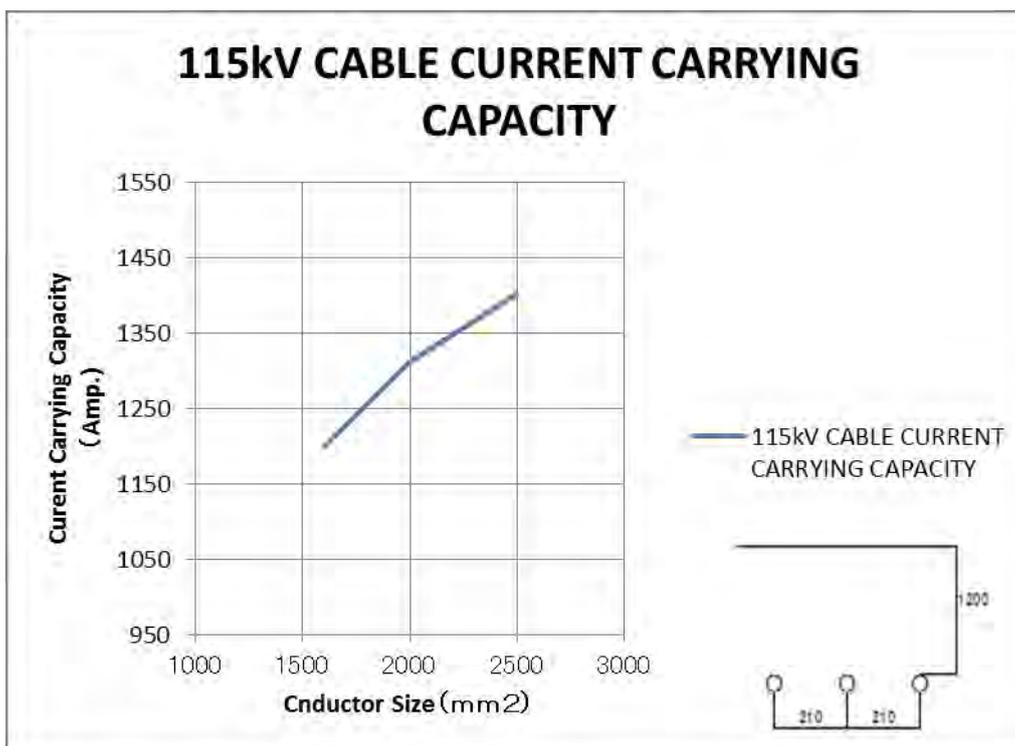
**Figure 6.6 Current Carrying Capacities of 115kV Underground Cables**
