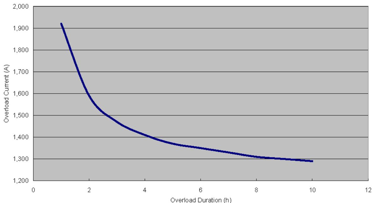
**Figure 3. 19 Short Term Capacity of Triplex-type 115kV Underground Cable**
