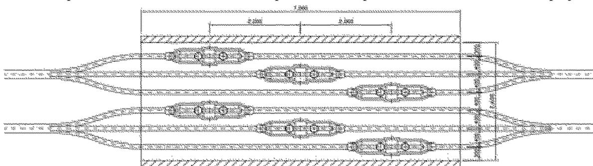
**Figure 7. 1 Typical Joint Arrangement**
