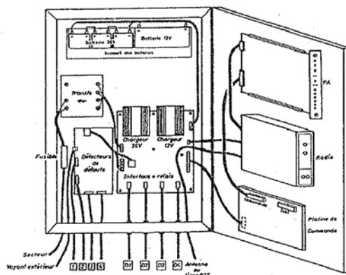
**Figure 6. 24 Radio Transceiver Equipment on Distribution Substation Building**
