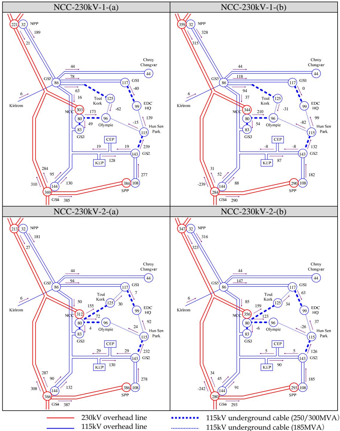
**Figure 3.25 Active Power Flow of the System with 230kV NCC Substation in 2020**
