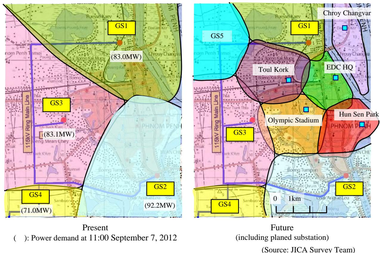
**Figure 3.16 Catchment Area of each Substation**
