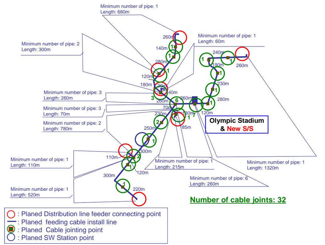
(b) Number of duct pipe and cable connection points
