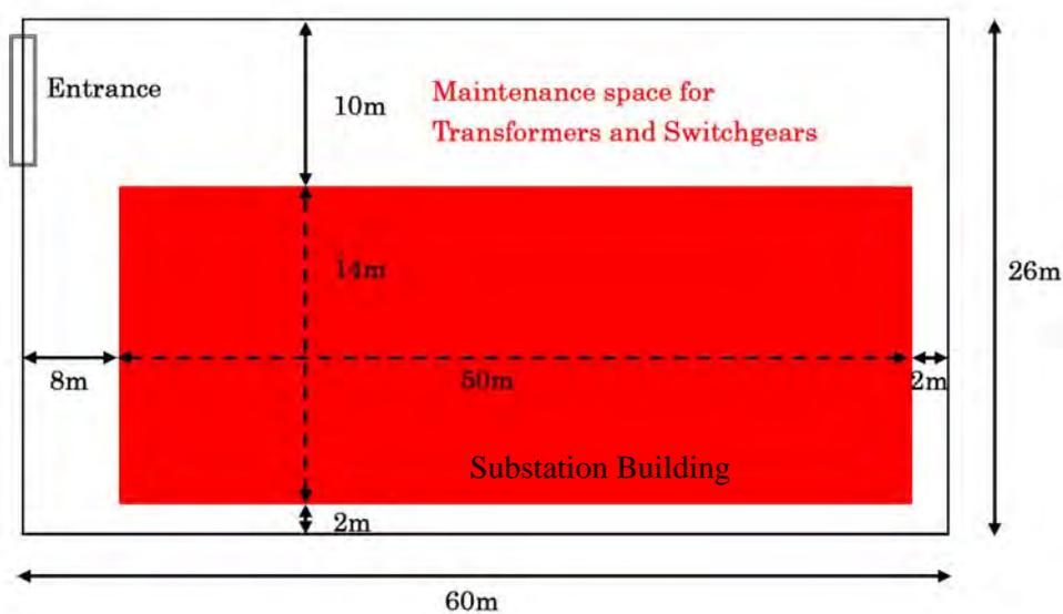
**Figure 6. 19 Allocation Image of Substation Building at Olympic Stadium Site**
