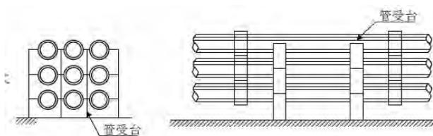
**Figure 6. 27 Example of Duct Pipe Layout**
