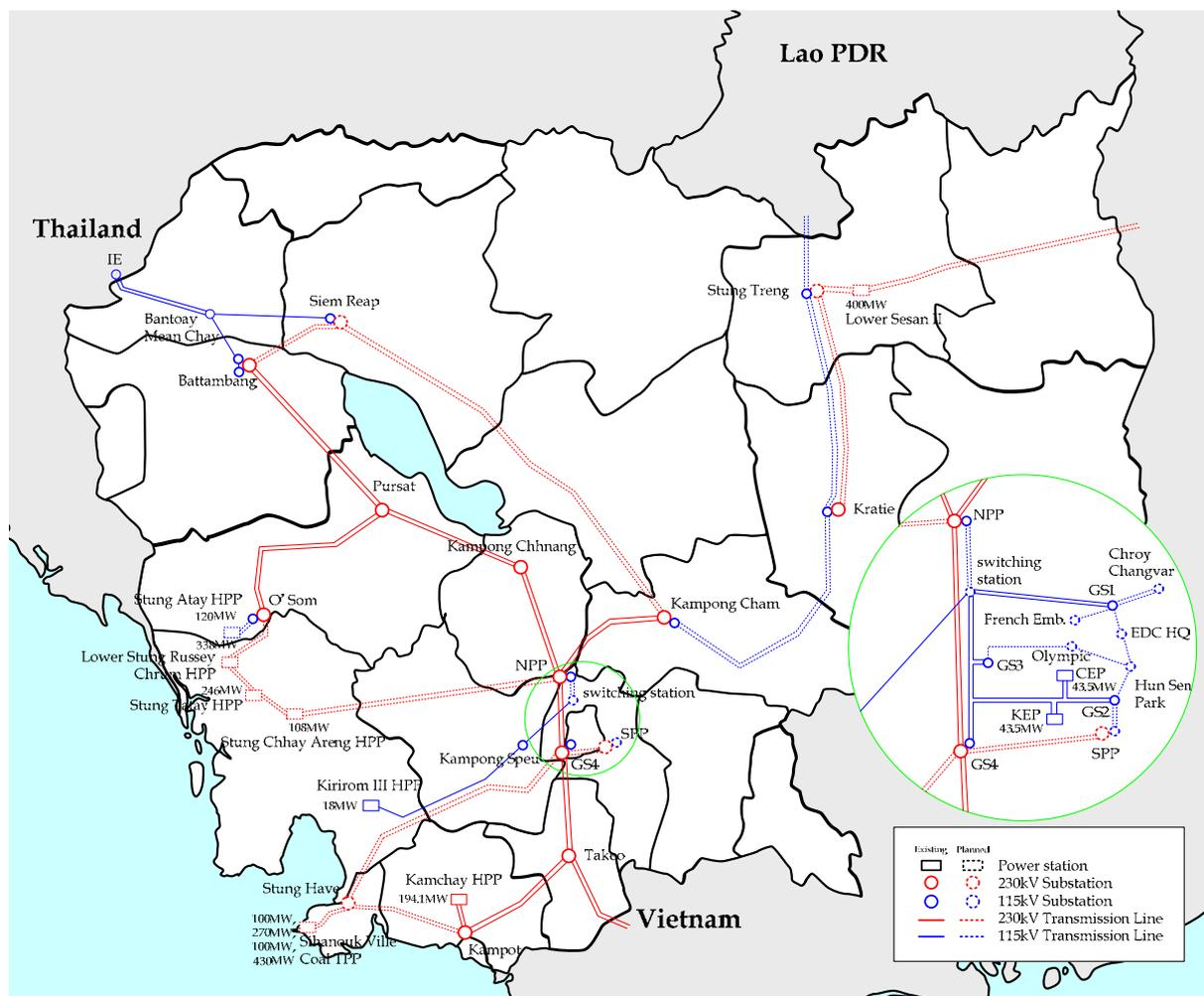
Figure 2. 17 Transmission system in Cambodia up to 2020
