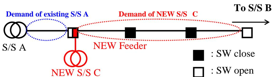
(a) New feeder connection and Load divides image of established distribution line
