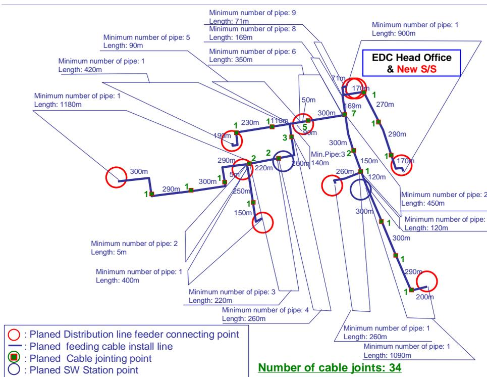
(b) Number of duct pipe and cable connection points
