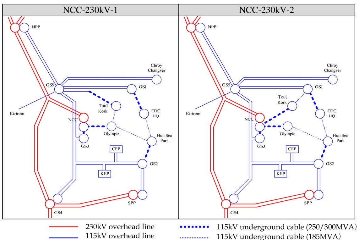
**Figure 3.24 Development of 230kV NCC Substation in 2020**
