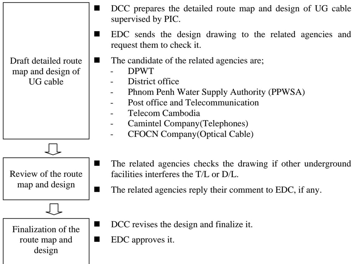
**Figure 8.2 Checking Procedure for underground facilities**
