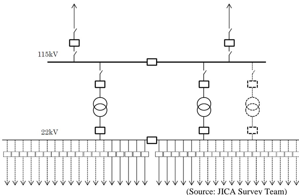
**Figure 6. 18 Single Line Diagram of Substation at Olympic Stadium**
