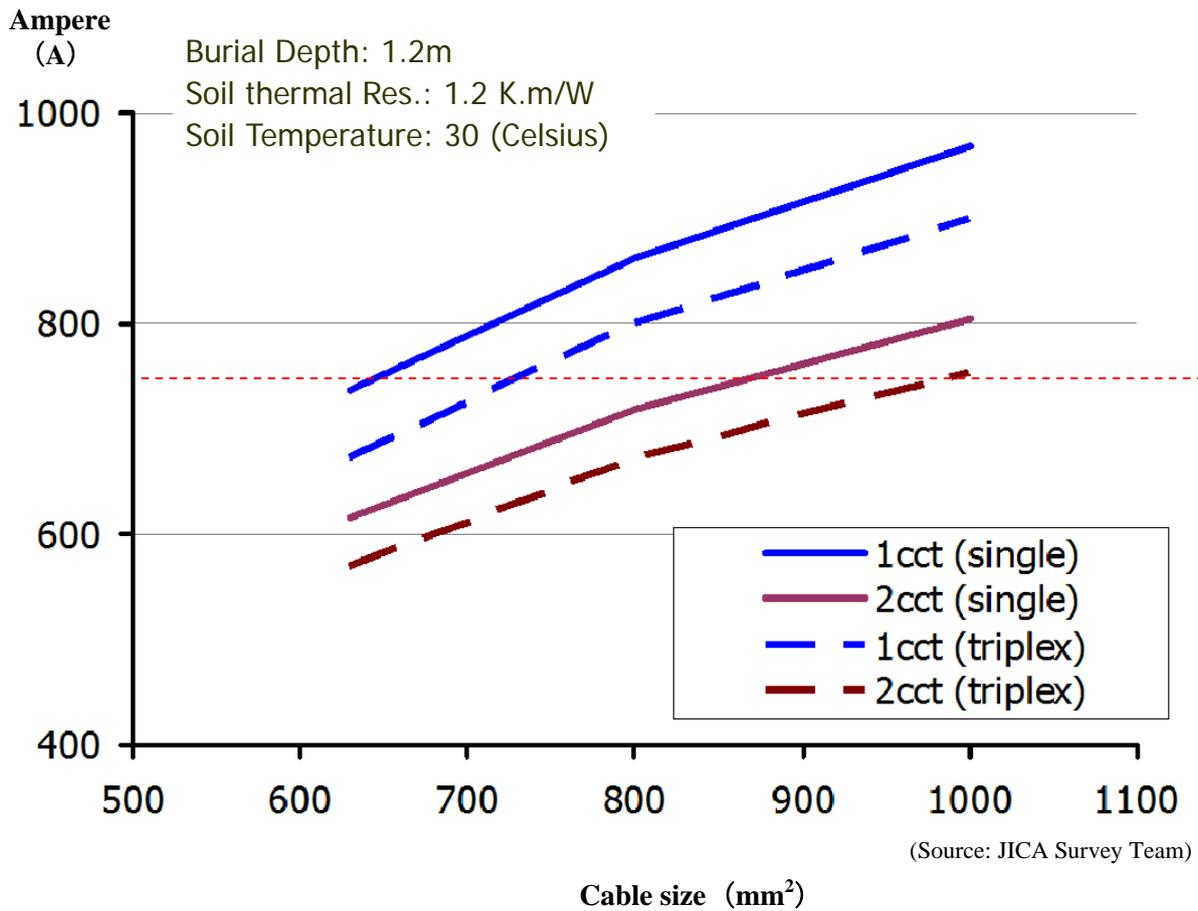
**Figure 6. 7 Current carrying capacity of single core and 3-core cables**
