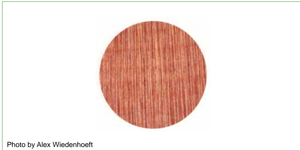
Figure E-2 Example of Araucaria araucana (Monkey puzzle tree) Wood Cross Section
