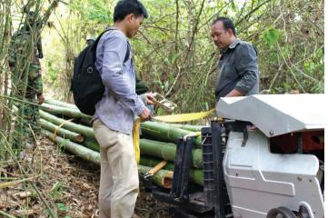
Ready for transport: the ForInfo bamboo crawler is loaded with over 350 kg's of fresh bamboo.
