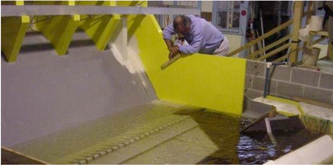
Figure 8-2. Example of a physical model of a 32 m high dam and fishway in Australia that was used to determine entrance location and hydraulic conditions for the fishway. Scale is 1:20 but 1:10 is preferred.
