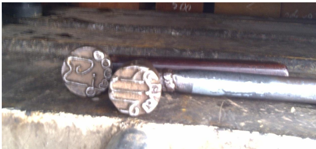
Figure 1. RFD staff marking hammers for logs and sawn timber.
