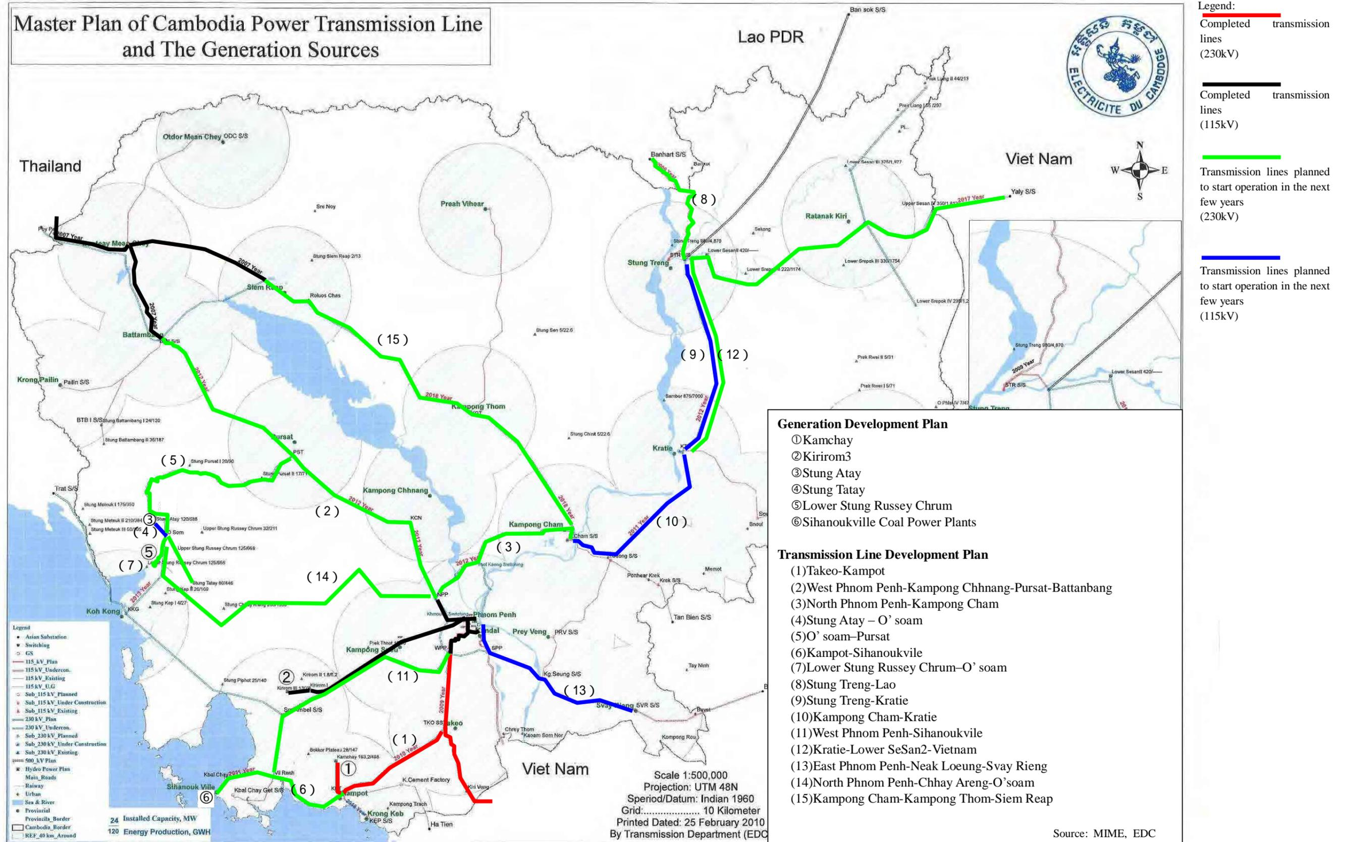
Figure 2-41 System structures and development plan
