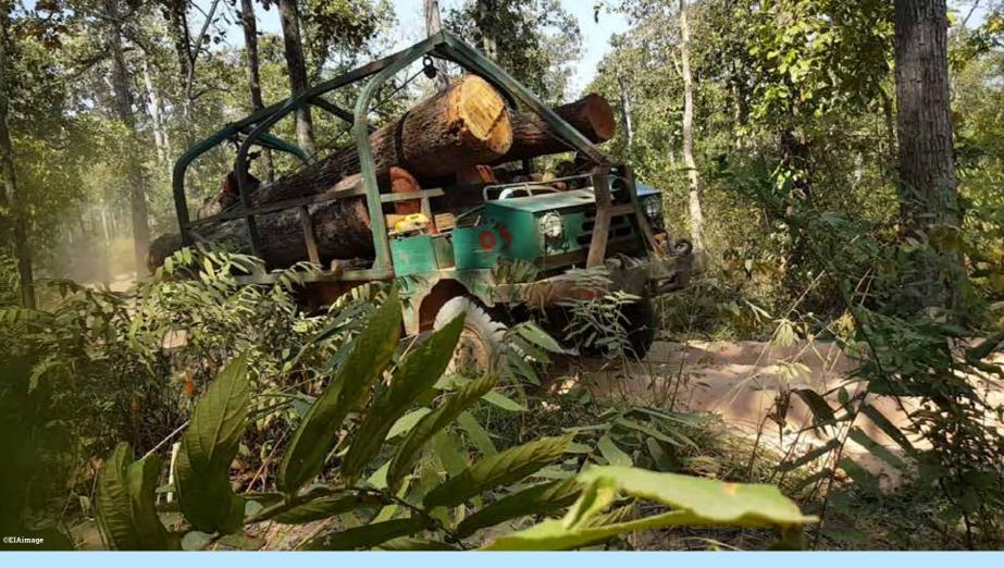
Above: Arevs are slow moving, basic trucks, capable of carrying up to 20m³ of logs along basic jungle tracks. Equipped with cranes, arevs can collect logs directly from felling sites
