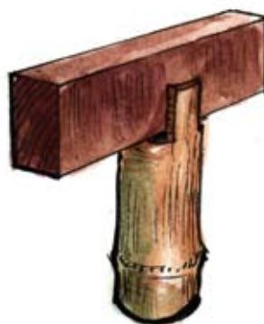
A possible bambo to wood joint.
