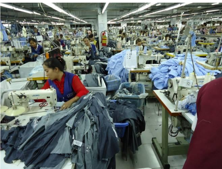
Access paths are not free of obstruction
