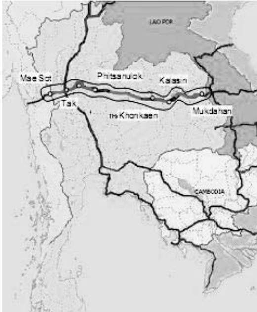
A. East-West Economic Corridor (R2) Myanmar-200 km Thailand-800 km: 50% is 4lanes Lao PDR-240km: 2 lanes Vietnam-260 km: 2 lanes
