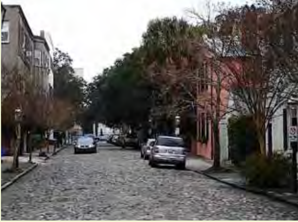
United States: Use of natural materials for residential street traffic calming in Charleston
