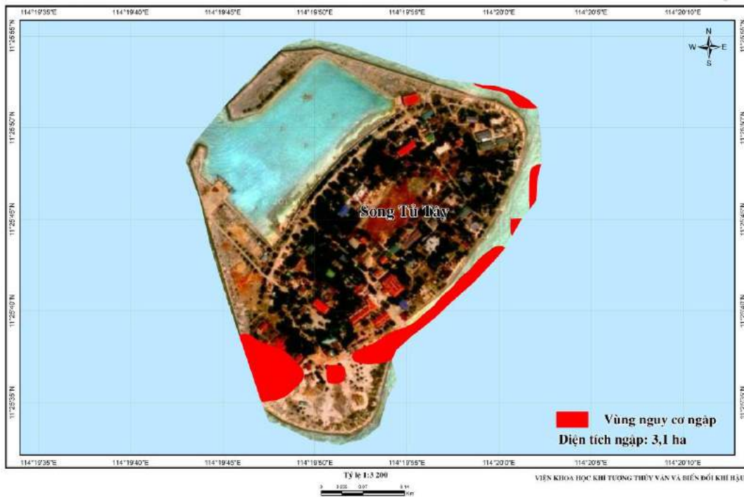
Figure B45. The inundation risk map with sea-level rise of 100cm, Song Tu Tay island, Truong Sa island group, Khanh Hoa province
