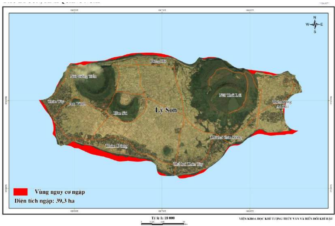
Figure B38. The inundation risk map with sea-level rise of 100cm, Ly Son island, Quang Ngai province
